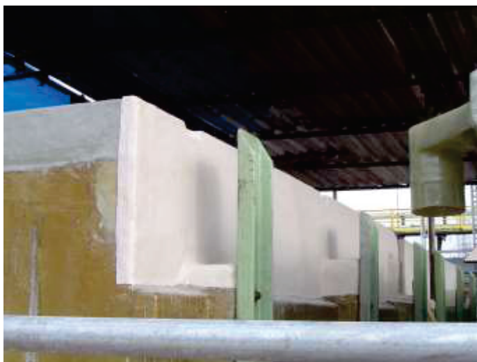
Electrolytic Cells in service after repair
